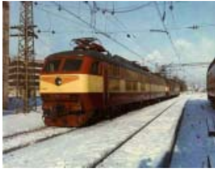
Electric locomotive capable of 8,000 KW output and a speed of 200 kph, built for the USSR (1977)
