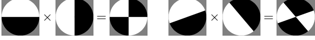
Figure 2: Creation of a checkerboard pattern as product of two individually rotated idealized edges. If black corresponds to -1 and white to 1 , this construction principle does not only hold for \phi = 0^\circ and \phi_2 = 90^\circ (left), but also for arbitrary angles like \phi_1 = 20^\circ and \phi_2 = 130^\circ (right).
